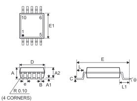
**Dimensions in inch** Symbol Min. Nom. Max. А \_\_\_\_ \_ 0.043 0.006 A1 0.000 \_ A2 0.030 0.033 0.037 0.007 0.013 b — 0.003 \_ 0.009 С \_ D \_ 0.118 BSC Е 0.193 BSC \_ \_ E1 0.118 BSC — \_ 0.020 BSC е \_ \_ L 0.016 0.024 0.031 0.037 BSC L1 \_ \_ 0.004 \_ у \_  $0^{\circ}$ \_ 8° α
