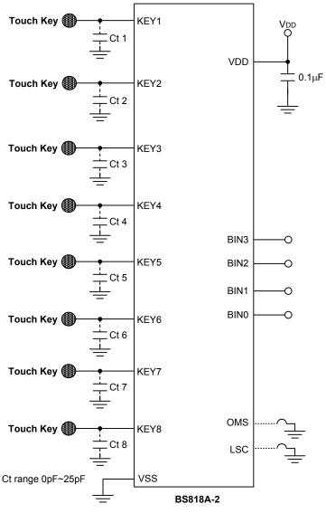
Note: 1. Ct (C threshold) is used for adjustment of Trigger Threshold. Recommended value: 0~25 pF
