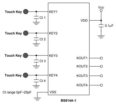
Note: 1. Ct (C threshold) is used for adjustment of Trigger Threshold. Recommended value: 0~25 pF
