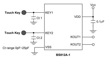
Note: 1. Ct (C threshold) is used for adjustment of Trigger Threshold. Recommended value: 0~25 pF
